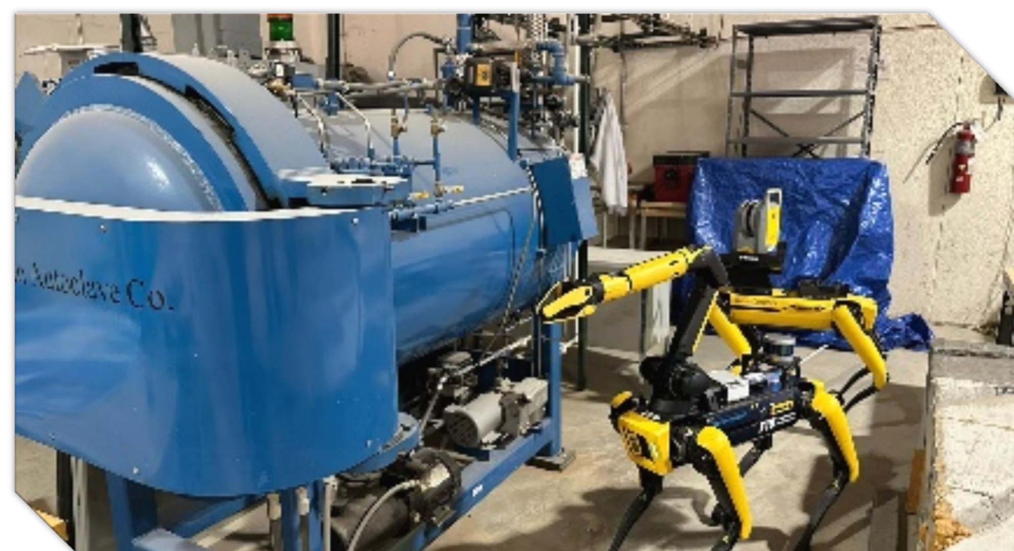
Robotic platform (SPOT) performing inspection in industrial DOE-relevant environment
